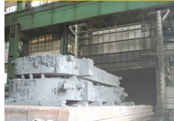
7m×14m heat treatment furnace
